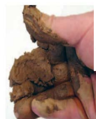
Lifting thumb from fingers to assess relative clay content (stickiness) — if the sample is too dry or too wet, stickiness (clay content) will be underestimated
