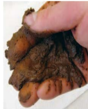
Rubbing sample hard to a thin film between the thumb and fingers to ensure all sand sizes are being assessed — if sample is not rubbed hard, sand content will be underestimated
